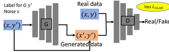
Fig. 2: Conditional GAN (CGAN) architecture:  $y'$  and noise vector  $\mathbf{z}$  are combined as input for generator  $G$ ,  $\mathbf{x}' = G(\mathbf{z}, y')$  is generated data,  $(\mathbf{x}, y)$  is real data-label pair,  $(\mathbf{x}', y')$  is generated data-label pair, discriminator  $D$  tries to distinguish generated data-label pair from real data-label pair, loss  $L_{CGAN}$  is given in Eq.(4).
