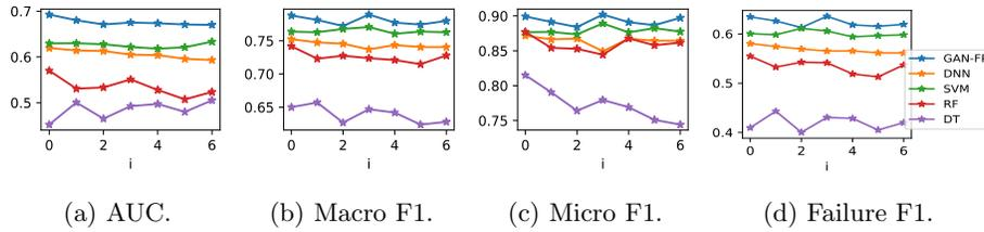
Fig. 7: CMAPSS FD001 class imbalance effect using GAN-FP and classifiers with SMOTE: in each figure, the x-axis  $i$  indicates  $(1000 * i)$  non-failure samples are randomly removed from the training data, we do not remove failure samples. The testing samples are fixed for all experiments.
