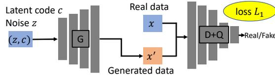
Fig. 1: InfoGAN architecture: latent code  $\mathbf{c}$  and noise vector  $\mathbf{z}$  are combined as input for generator  $G$ ,  $\mathbf{x}' = G(\mathbf{z}, \mathbf{c})$  is generated data,  $\mathbf{x}$  is real data, discriminator  $D$  tries to distinguish generated data from real data, network  $Q$  is used to maximize  $L_{mutual}$  (Eq.(2)), loss  $L_1$  is given in Eq.(3).
